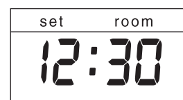
F: When the 4-digit stops blinking, the setting has been locked to the indicated value.
